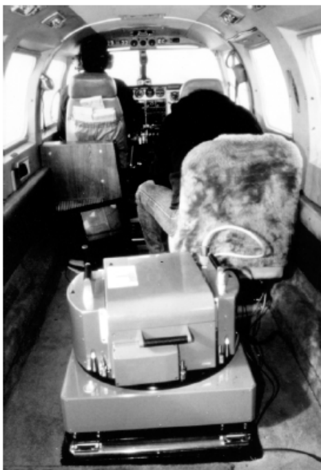
Typical aerial photographic installation. (Courtesy of Surdex Corporation, Chesterfield, MO.)
